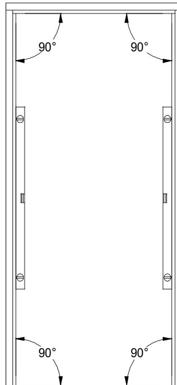
The positioning of installation fixings in height must be planned to avoid conflicts with the lock keeps, draught and intumescent fire seals.
