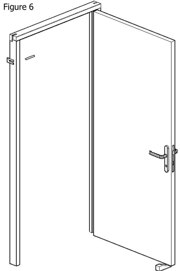
With the door almost closed, align the edge of the door with the edge of the frame, so that the gap is the same from the top to bottom of the door.
