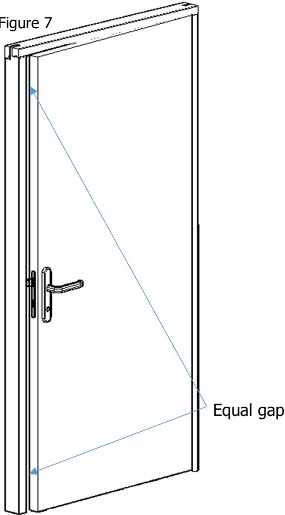
Repeat this procedure after each frame fixing point, this will allow for any possible bow or twist of the door leaf.
