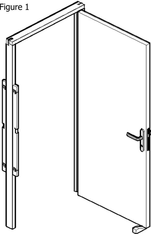
Place the door and frame in structural opening and then open the door 90 degrees. Position a suitable packer beneath the opening edge of the door leaf, ensure the hinge side of the frame is plumb to both internal and external faces using a spirit level.
