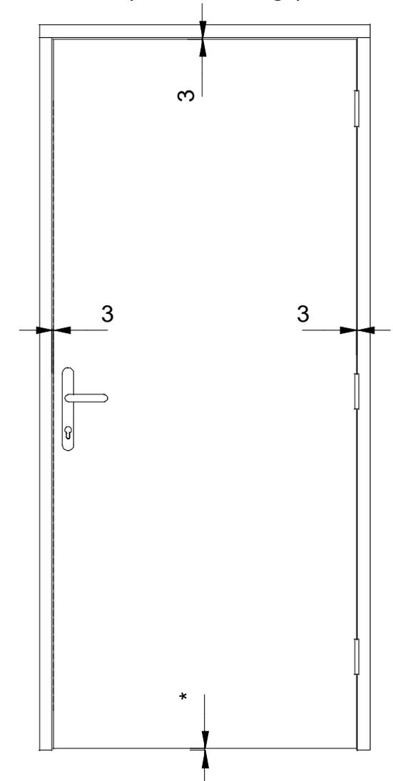
Apply an intumescent mastic sealant between the frame and the structural opening all around the frame.
