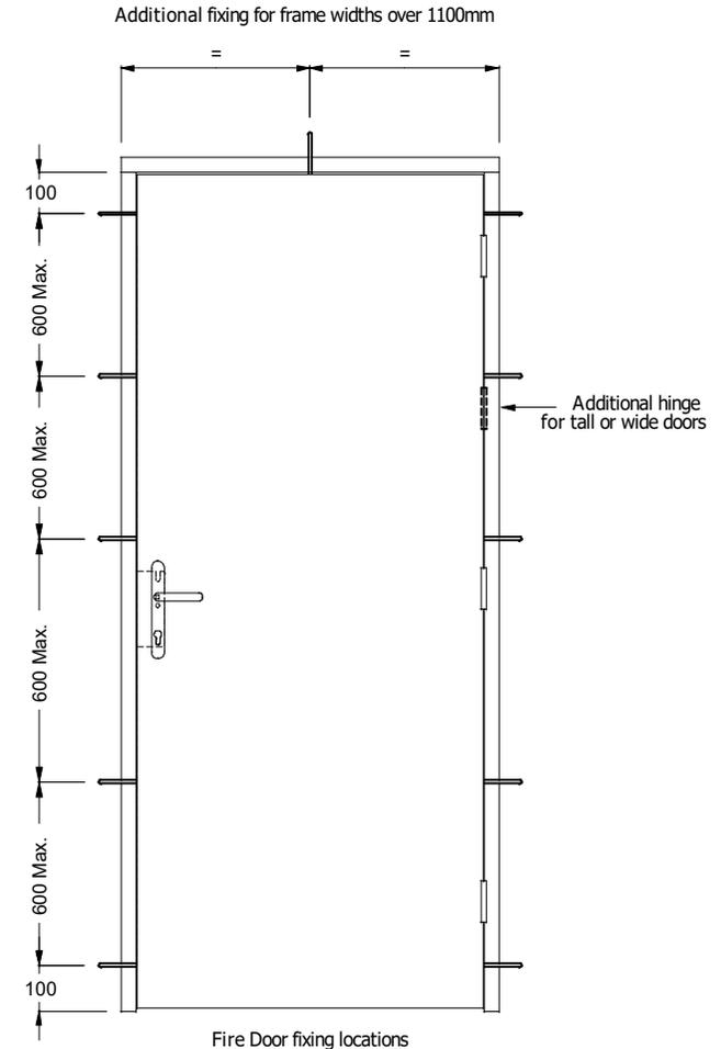
Ensure that frame is plumb, before fixing the hinge side of the door
